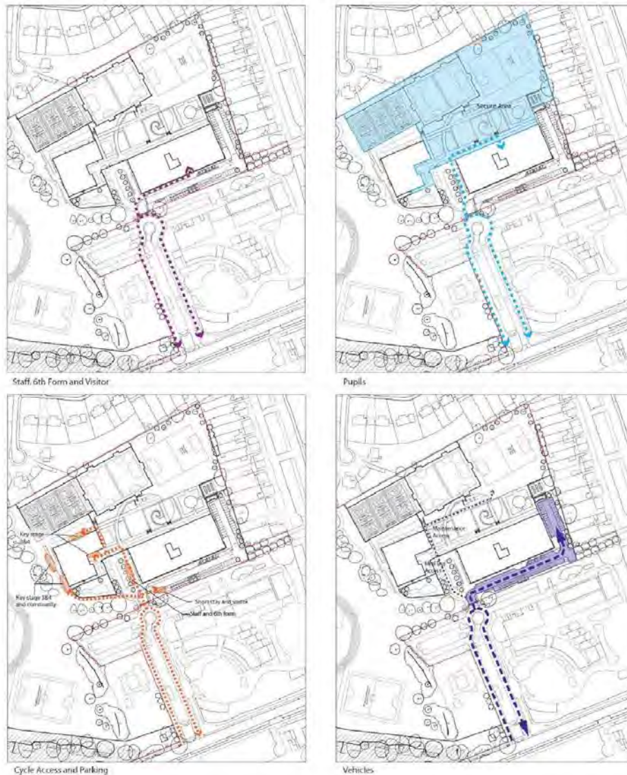
Figure 3 Site Layout, Movement & Access Arrangements
